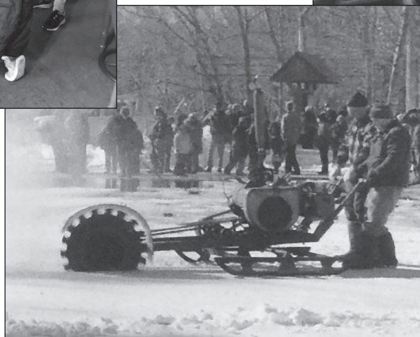
The restoration of our own 1919 Novice ice saw is ending thanks to the work of board member Bill Wilkins and volunteer Cal Mc-Graw. It still needs its blade sharpened while the pouring of a set of new babbit bearings is underway.
